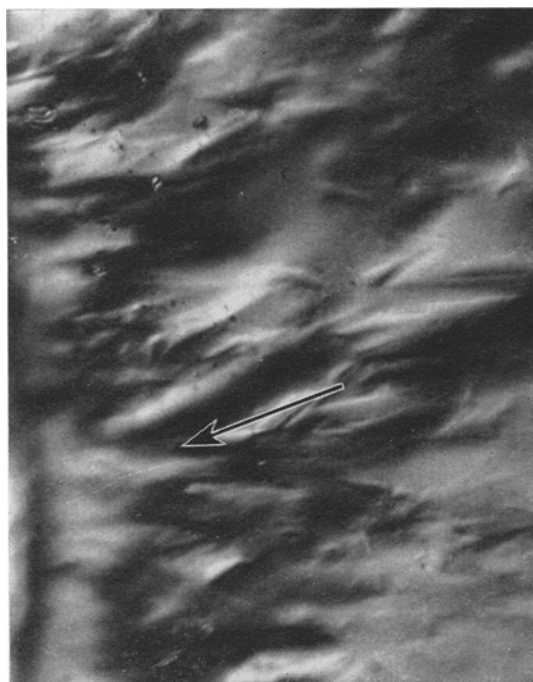
Figure 1 Two-stage etch (stage 1). Smooth SiC coat. Nomarski interference contrast. Deposition direction – see arrow. ( \times 610 – reduced from \times 780 for reproduction)
